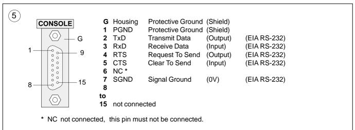
Fig. 7: Terminal assignment of the serial interface CONSOLE
