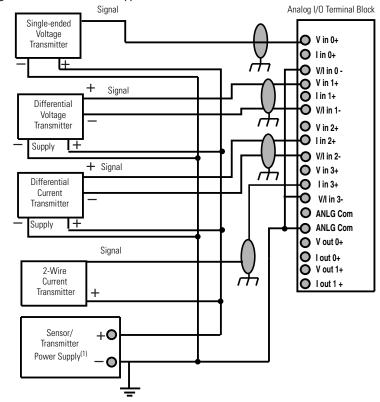
(1) The sensor power supply must be rated Class 2.
