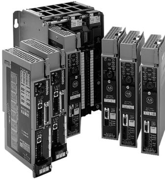
Every PLC-5 controller offers built-in, configurable ports for Data Highway Plus (DH+) or Universal Remote I/O. A DH+ connection supports remote programming and information access, in addition to peer-to-peer communication between the PLC-5, other controllers and devices. A Universal Remote I/O connection supports real-time data exchange for I/O, operator interface, and other third-party devices.
