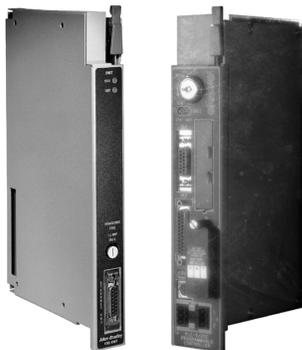
The PLC-5 Ethernet Interface Module (1785-ENET) is a single-slot module that attaches to the side of any Enhanced PLC-5 series B or later controller, Ethernet PLC-5 controller, or ControlNet PLC-5 controller to provide additional Ethernet connectivity.
