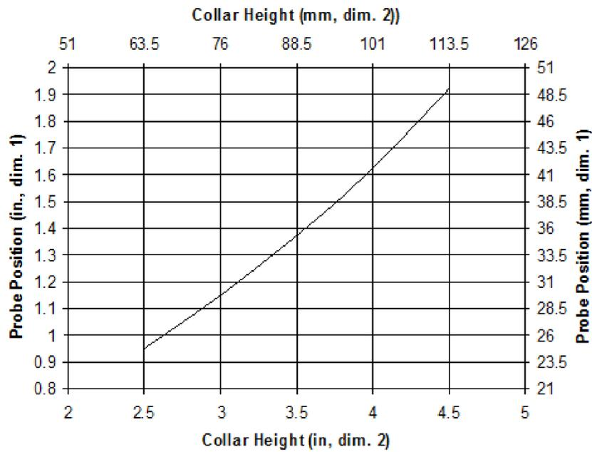
**Figure 9: Recommended Probe Position Based on Collar Height**
