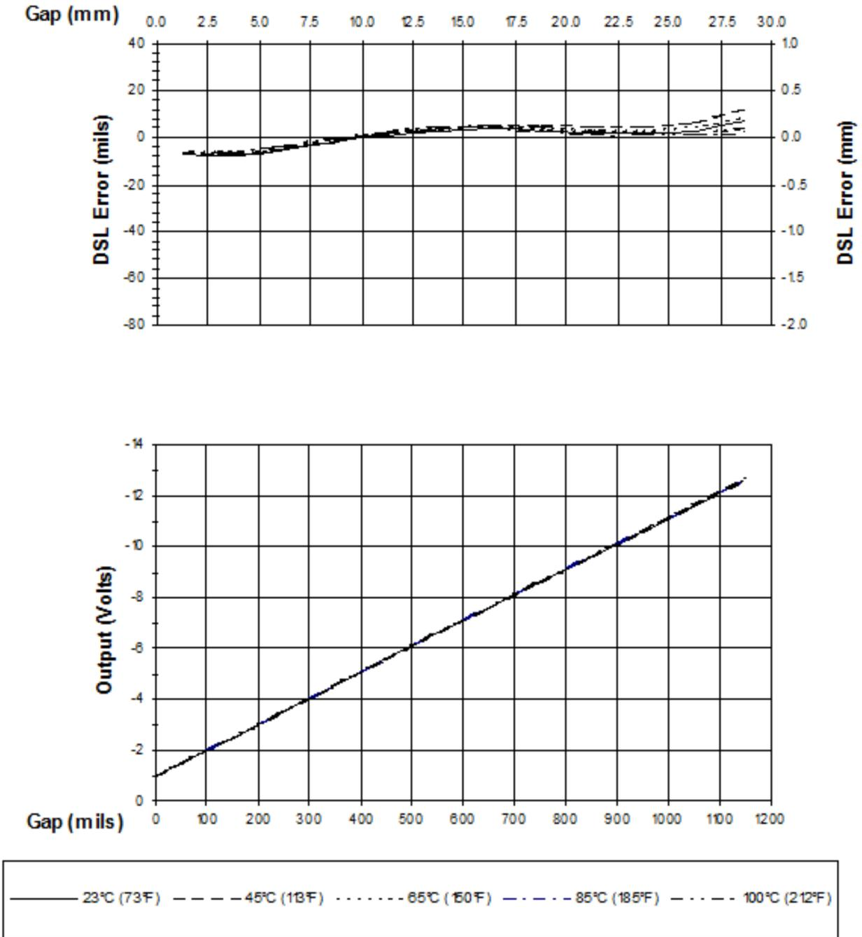
**Figure 8: Typical 3300 XL 50 mm 9 m Proximito with 8 m of Extension Cable @ High Temperature (Probe is at 25°C.)**
