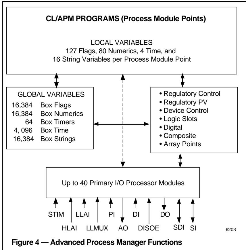
Figure 4 — Advanced Process Manager Functions
