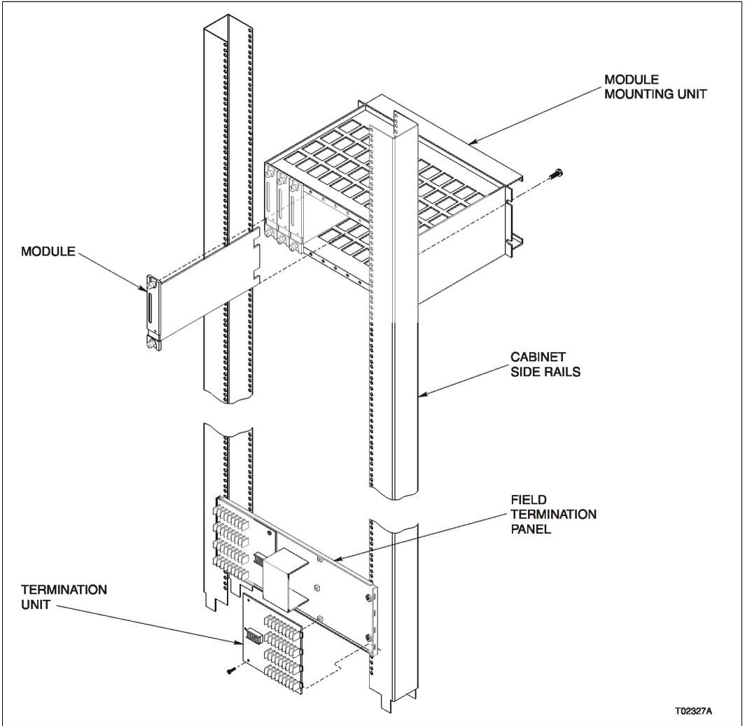
**Figure 2-6. Mounting Hardware**
