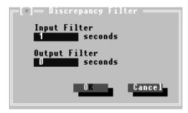
The output discrepancy filter can be set to increase the time interval needed to detect an output discrepancy. This time defaults to 0 seconds.
