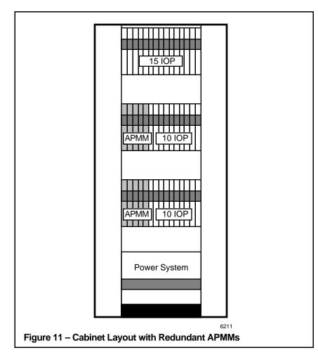
Optional power redundancy and battery backup can be provided for assured power availability.
