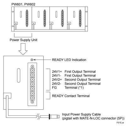
\*1: When you use PW60 installed on ACB41, or use PW60 with AEP7D, the FG terminals need not be connected.
